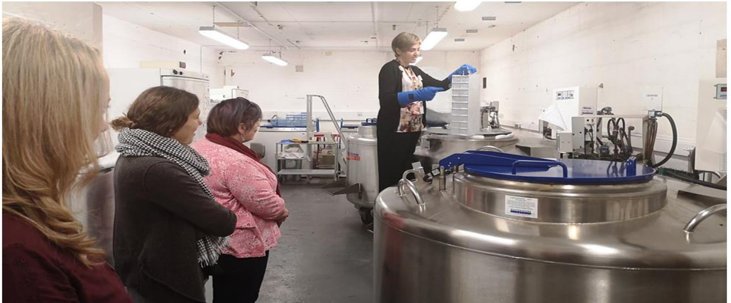
*Fragile biological samples are preserved in these tanks by cooling them to very low temperatures using liquid nitrogen*
